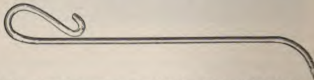
Fig. 279.—Needle specially designed to carry a thick wire. The eye is drilled obliquely, and should receive only a little loop on the end of the wire; this loop should be made previously.
